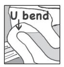
A new pipe was invented in 1775. This pipe is shaped like a U. This pipe traps the smelly water. This pipe is still used today. This pipe made people want a flushing toilet.
